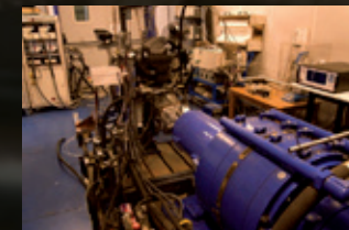
2 fully equipped engine benches for emissions testing
